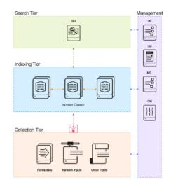
The basic topology consists of a Search Head running out of the box, untuned Enterprise Security; a clustered indexing tier with a non-indexing Master Node; a License Master; and one (1) or more Universal Forwarders generating sample data to send to the index cluster. Because this environment operates on Kubernetes and uses the Splunk support Ansible playbooks, all apps are deployed when the containers are built, and thus no Deployment Server is used.
